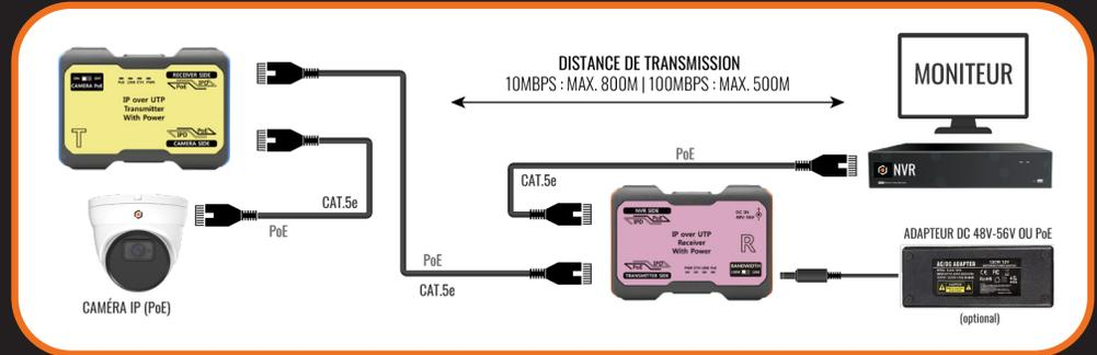
TRANSMETTEUR DE DONNÉES EN RÉSEAU - SOLUTION DE TRANSMISSION VIA CABLE UTP
