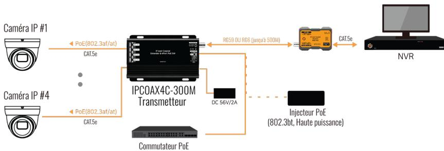
TRANSMETTEUR DE DONNÉES HYBRIDE IP SUR COAXIAL - CONNECTEZ JUSQU'À 4 CAMÉRAS À 500M
