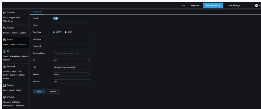
The screenshot shows the 'Event Push' configuration page in a web interface. The 'Enable' toggle is turned on. The 'Push Way' is set to 'HTTP'. The 'Method' is set to 'POST'. The 'Interval' is set to 'OFF'. The 'Server Address' is '192.168.1.103 or example.com', the 'Port' is '123', and the 'URL' is 'APIAlarmEventEventPush'. There are 'Save' and 'Refresh' buttons at the bottom.
