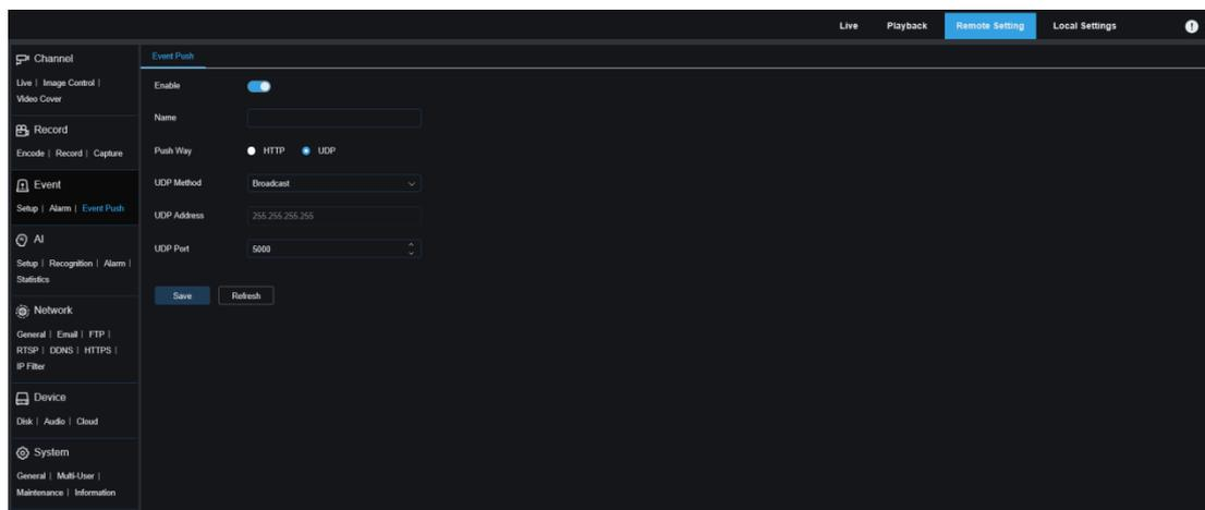
The screenshot shows the 'Event Push' configuration page in a web interface. The 'Enable' toggle is turned on. The 'Push Way' is set to 'UDP'. The 'UDP Method' is set to 'Broadcast'. The 'UDP Address' is '255.255.255.255' and the 'UDP Port' is '5000'. There are 'Save' and 'Refresh' buttons at the bottom.
