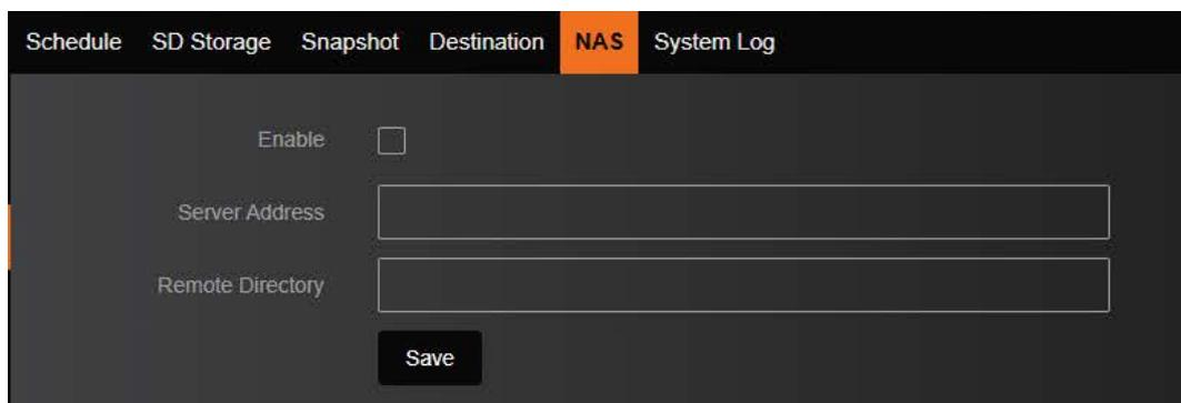
**Server Address**-- IP address of NAS network hard disk.
