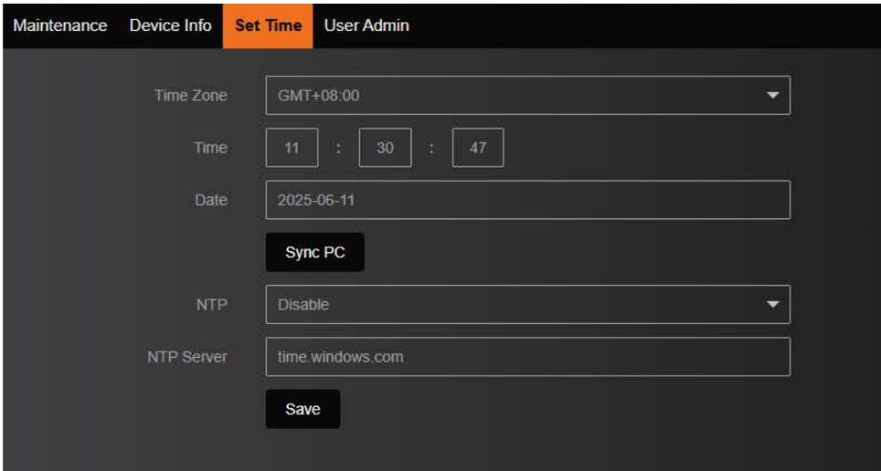
**Time Zone**-- The time zone shows the current time zone of the device and it can be modified according to the actual situation.
