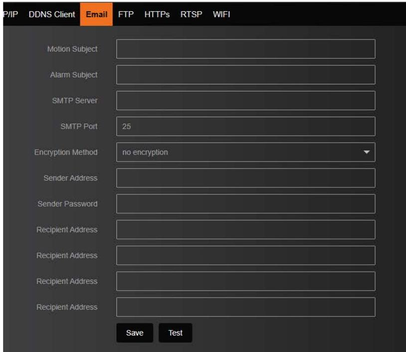
The screenshot shows a settings menu with tabs for P/IP, DDNS Client, Email, FTP, HTTPs, RTSP, and WIFI. The 'Email' tab is selected. The configuration fields include: Motion Subject, Alarm Subject, SMTP Server, SMTP Port (set to 25), Encryption Method (set to no encryption), Sender Address, Sender Password, and four Recipient Address fields. At the bottom, there are 'Save' and 'Test' buttons.
