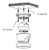
Fi x the pedestal by drilling locking holes around the sticker and inserting three expansion bolts into the holes and fastening it with three locking screws.
