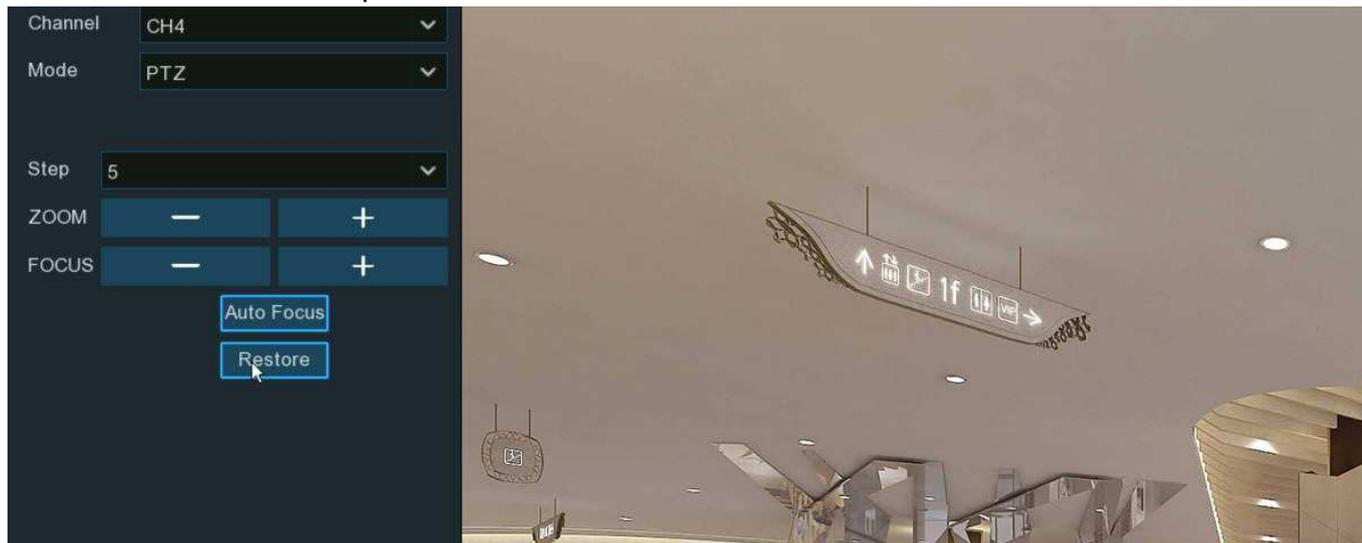
**Step:** To set the steps of each movement of the MFZ lens
