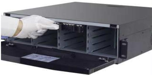
(4) Buckle up the hard disk and close the front panel.
