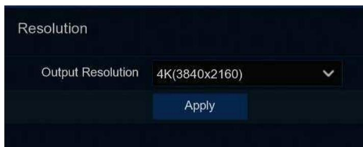
If you connect to a 4K HDMI monitor, you are able to choose max. 4K (3840x2160) resolution. If you connect a VGA monitor, do not choose the resolution larger than 1080P(1920x1080).
