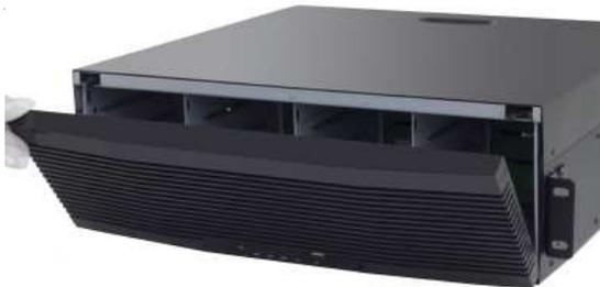
Align the hard disk slot and then insert the hard disk gently and smoothly.
