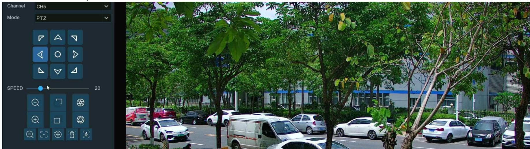
**Mode:** To control the PTZ camera by PTZ, Preset, Line Scan, Watch Mode, Tour and Pattern Scan.
